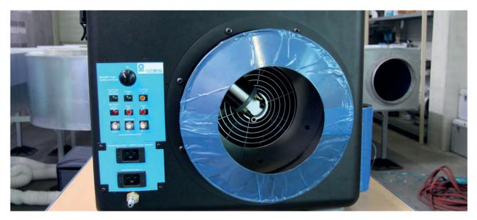
The Aeroseal machine heats up the sealant and blows it into the duct as a fog. The fog will then seal the holes and leakages from inside the duct.
