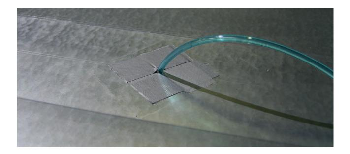
Duct pressure is measured throughout the process to give real-time sealing data.
